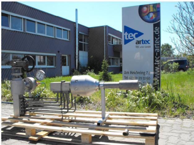
Siemens/Vienna and Beuth University/Berlin, a new multistage controlled superheated steam attemperator (desuperhater) without any movable parts in the steam tube. This new development called TECtemp HT gets realized at the RWE power plant in Ibbenbüren, in progress of a planned revision, for the first time.
